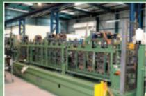
Servo controlled steel framing line.
