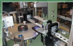
Special purpose feeding equipment for water filter manufacture.
