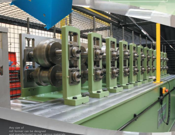
Any size of roll former can be designed and manufactured to suit various materials from 0.4mm - 6mm thick up to 1500mm wide.
