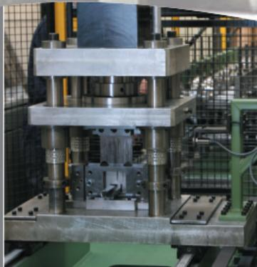
"Flying" cut offs can be integrated into the line as well as pre-piercing, bending and welding.
