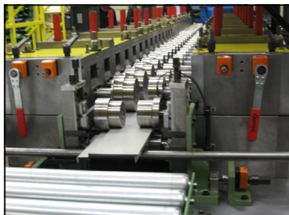
**28 Pass Duplex CNC Rollformer for the Production of Modular Building Panels (150-1000 Wide)**
