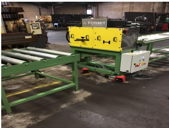
**I-Beam Post Chamfer & Slot Punching System.**
